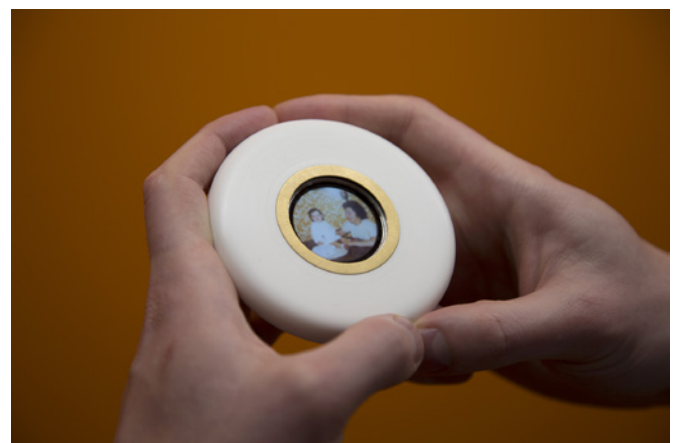
ReFind piece made from Corian®, brass and an android digital watch (designed and made by Trevor Duncan and Jayne Wallace, coding by Kyle Montague and Luis Carvalho).
